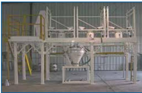
This system was designed for a company that produces industrial floor coverings. APEC provided the bulk bag dischargers, micro scale, tote staging system, bag dump station, and complete automation including motor control center and computer based recipe automation.
